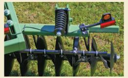
Spring cushion models of the Wishek Tandem Disc offer unique flexibility in their design. When a blade strikes a solid object, it travels in an arc of 12 inches (305 mm) rearward and upward, letting it travel over and avoid damage from impact with that object.
