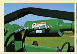
An adjustable leveling system is standard equipment, allowing unit to be leveled front to back. An optional hydraulic leveler is available (shown).
