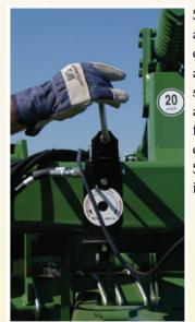
Single-point depth control allows the operating depth of the entire disc to be adjusted with a single setting. This simple adjustment, done at the front of the machine, is easy, safe, and precise. Single-point depth control is optional on all models.
