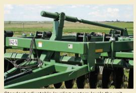
Standard adjustable leveling system levels the unit front to rear. A hydraulic leveler is optional.
