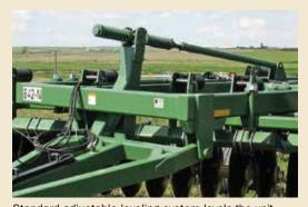
Standard adjustable leveling system levels the unit front to rear. A hydraulic leveler is optional.
