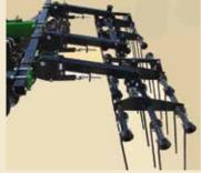
To assist in leveling the field and help create a better seedbed, add a 3-bar harrow. The tubular tooth bar harrow features % x 26 inch tines (16 x 660 mm) for strength and durability.
