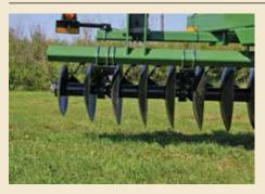
Wishek 812N-OCL Offset Disc features 28 inch (711 mm) blades on 11 inch (279 mm) spacing. The winged model comes with an OCL (Over Center Lock) system for complete leveling performance. The OCL system on the 812N unit prevents the disc wings from diving or lifting out of the ground by locking the wings rigid to the main frame.
