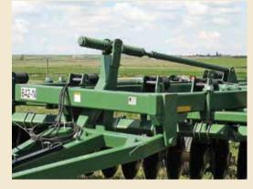
Standard adjustable leveling system levels the unit front to rear. A hydraulic leveler is optional.
